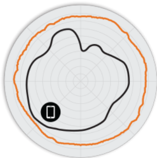
Figure 2. T300 2.4GHz Azimuth Antenna Patterns
