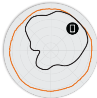
Figure 3. T300 5GHz Azimuth Antenna Patterns
