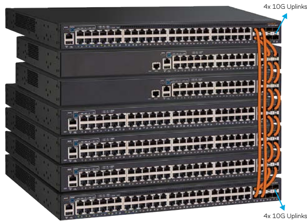
Figure 1: Up to 12 RUCKUS ICX 7150 Switches can be stacked together using up to four SFP+ 10 Gbps ports per switch for a fully redundant backplane delivering 480 Gbps of aggregated stacking bandwidth.
