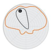
Figure 5. R750 5GHz Elevation Antenna Patterns
