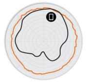
Figure 3. R750 5GHz AzimuthAntenna Patterns
