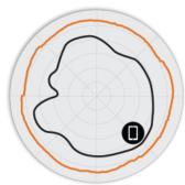
Figure 4. R750 2.4GHz Elevation Antenna Patterns
