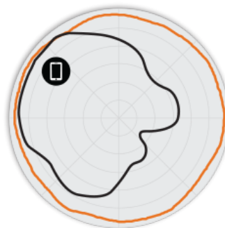
Figure 3. R710 5GHz Azimuth Antenna Patterns
