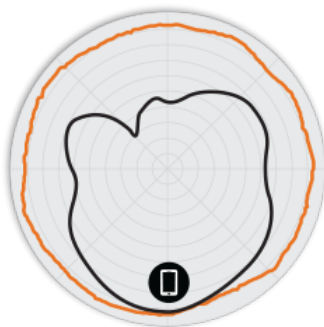
Figure 2. R710 2.4GHz Azimuth Antenna Patterns
