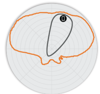
Figure 5. R710 5GHz Elevation Antenna Patterns
