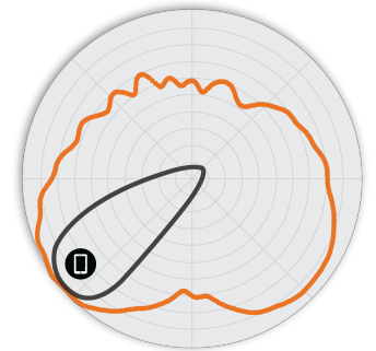
Figure 5. R550 5GHz Elevation Antenna Patterns
