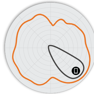
Figure 4. R550 2.4GHz Elevation Antenna Patterns
