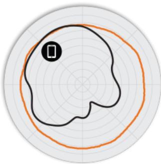
Figure 2. H510 2.4GHz Azimuth Antenna Patterns
