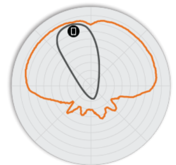
Figure 5. H510 5GHz Elevation Antenna Patterns
