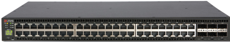
Figure 2. The Brocade ICX 7750-48C features 48 10GBASE-T ports and 6 40 GbE QSFP+ ports that can each be split into 4×10 GbE SFP+ ports.
