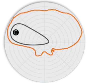
Figure 5. T750 5GHz Elevation Antenna Patterns
