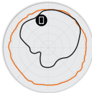
Figure 3. T301n 5GHz Azimuth Antenna Patterns
