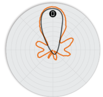
Figure 5. T301n 5GHz Elevation Antenna Patterns
