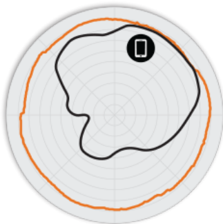
Figure 2. T301n 2.4GHz Azimuth Antenna Patterns
