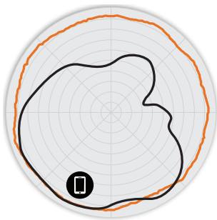
Figure 2. R700 2.4GHz Azimuth Antenna Patterns
