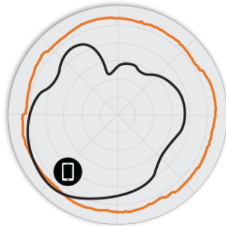
Figure 3. T710o 5GHz Azimuth Antenna Patterns
