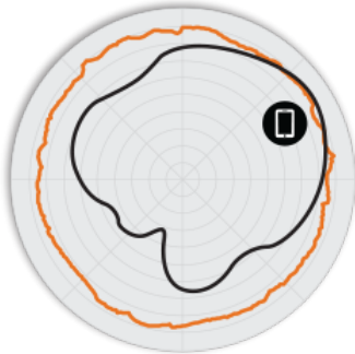
Figure 2. T710o 2.4GHz Azimuth Antenna Patterns
