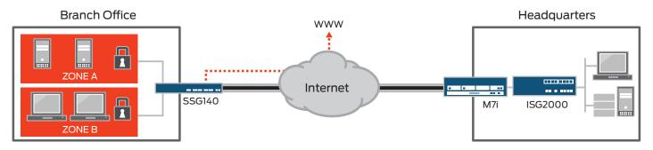
The SSG140 deployed at a branch office for secure Internet connectivity and site-to-site VPN to corporate headquarters. Internal branch office resources are protected with unique security policies for each security zone.
