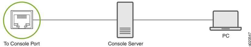
**Figure 46: Connect a Device Directly to a Management Console**
