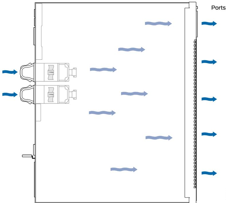
Under normal operating conditions, the fans operate at moderate speeds for minimal noise. Temperature sensors in the chassis monitor the temperature within the chassis. If any fan fails or if the temperature inside the chassis rises above the threshold, the switch raises an alarm and all functioning fans operate at a higher speed than normal. If the temperature inside the chassis rises above the threshold, the switch shuts down automatically.
