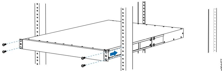
8. Have a second person secure the front of the switch to the rack by using the appropriate screws for your rack.
