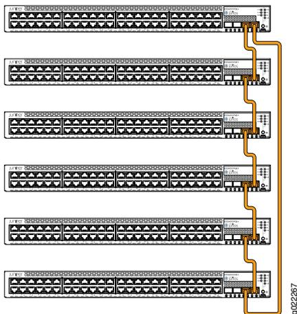
Figure 22: EX3400 Switches Mounted on a Single Rack and Connected in a Ring Topology: Example 2
