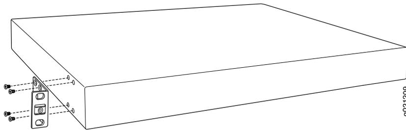
**NOTE:** If you need to mount the switch in a recessed position, use the 2-in.-recess front-mounting brackets from the separately orderable four-post rack-mount kit.
