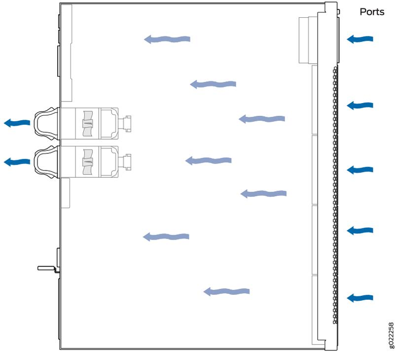
Figure 18: Back-to-Front Airflow Through the EX3400 Switch Chassis
