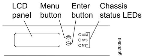
Figure 50: LCD Panel in an EX4300 Switches Except EX4300-48MP and EX4300-48MP-S Switches
