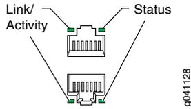
Figure 8: LEDs on the SFP+ Uplink Ports
