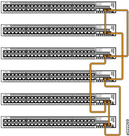
Figure 24 on page 89 and Figure 25 on page 90 show six EX3400 switches mounted on the top rows of adjacent racks and interconnected in a ring topology.
