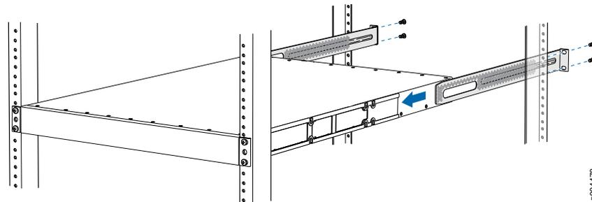
10. Attach the rear-mounting blades to the rear post by using the appropriate screws for your rack. Tighten the screws.
