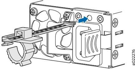
Figure 39: Connecting an AC Power Cord to the AC Power Cord Inlet
