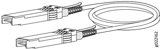
The cables are hot-removable and hot-insertable: You can remove and replace them without powering off the switch or disrupting switch functions. A cable comprises a low-voltage cable assembly that connects directly into two 10-Gigabit Ethernet ports, one at each end of the cable. The cables use high-performance integrated duplex serial data links for bidirectional communication and are designed for data rates of up to 10 Gbps.
