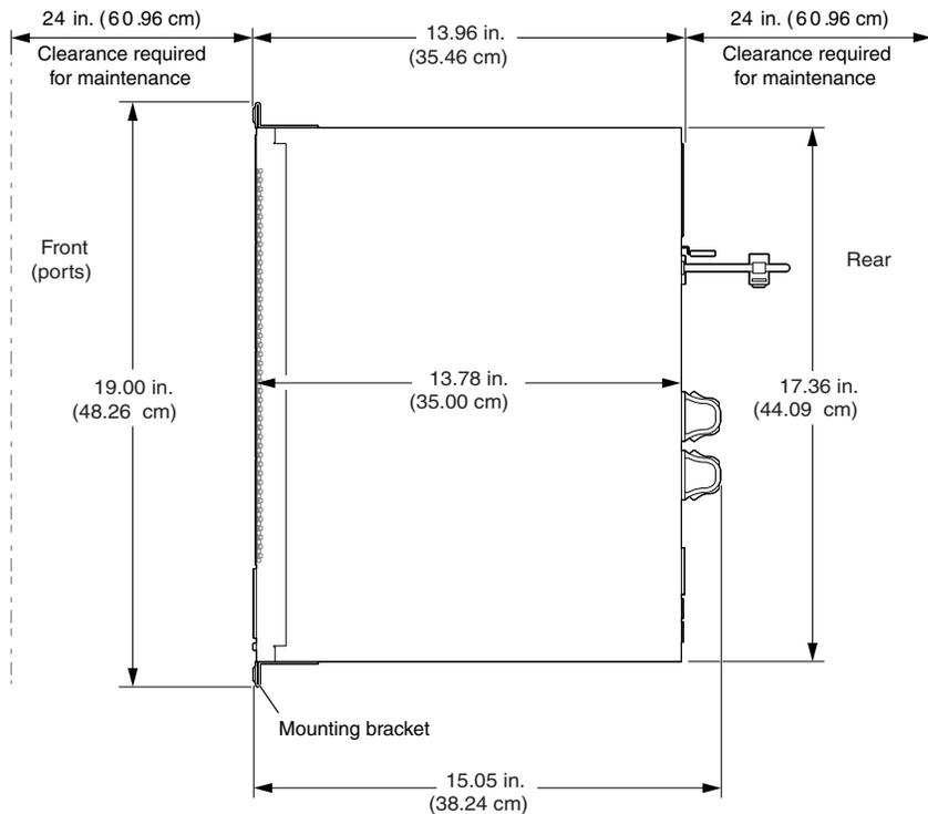
The power cord retainer extends out of the rear of the chassis by 3 in. (7.62 cm). The fan module handle extends out of the chassis by 1.2 in. (3 cm).
