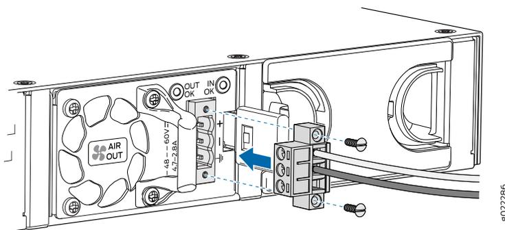
**NOTE:** To supply sufficient power, terminate the DC input wiring on a facility DC source that is capable of supplying a minimum of 7.5 A at -48 VDC.
