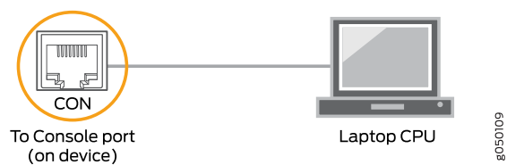
Figure 168: Connecting the QFX Series Directly to a Management Console
