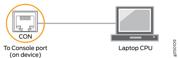
Figure 186: Connecting the QFX Series Directly to a Management Console
