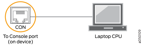
Figure 152: Connecting the QFX Series Directly to a Management Console
