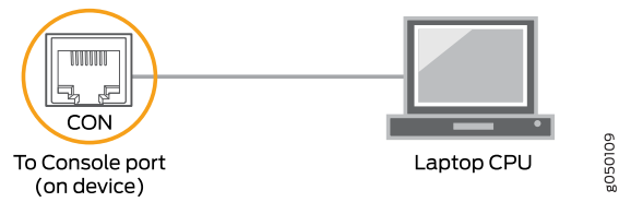
Figure 207: Connecting the QFX Series Directly to a Management Console
