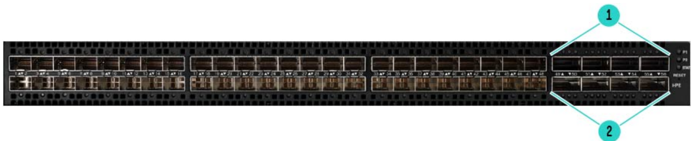
HPE Composable Fabric Rack Connectivity Module – Access Ports
