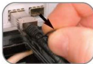
Figure 2. Disconnecting Latch Mechanism
