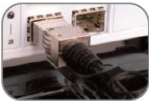
Figure 1. Installing an SFP+ Module
