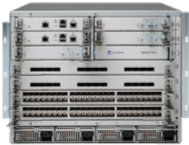
Figure 1: The VDX 8770-4 Switch supports up to 192 10 GbE ports, 108 40 GbE ports, and 24 100 GbE ports.
