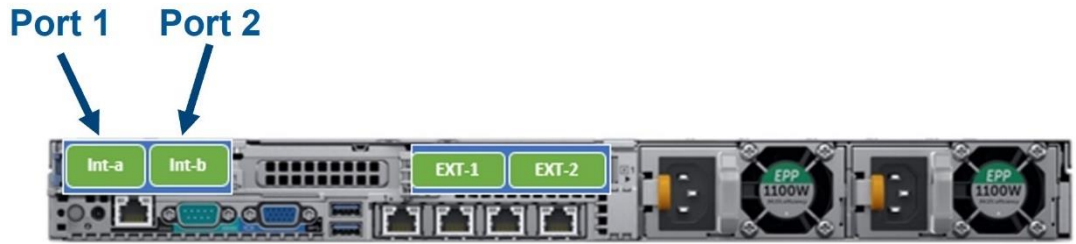
Figure 3. F600: back-end ports
