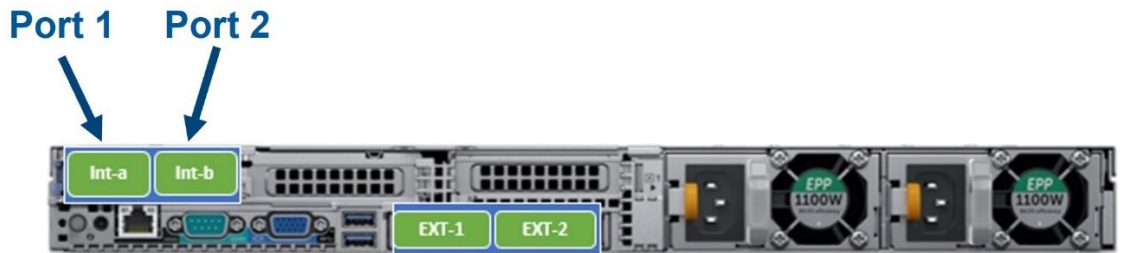
Figure 2. F200: back-end ports
