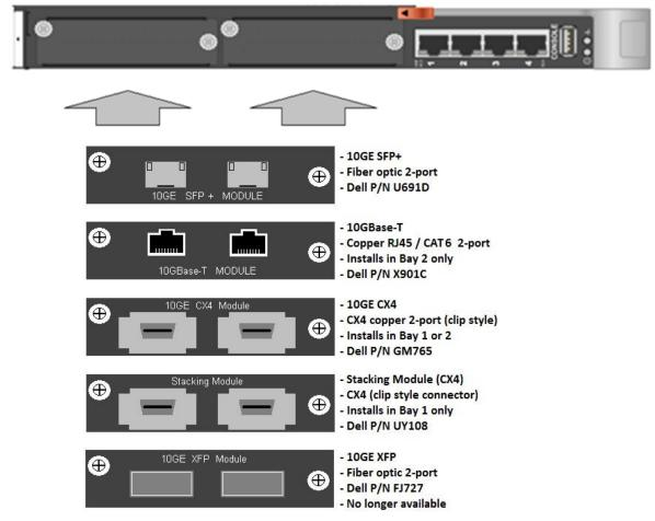
Figure 4 Dell Networking M6220 Blade Switch (1G Ethernet) and Available Modules
