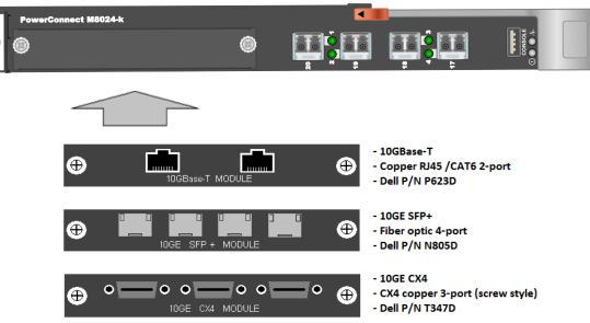
Figure 2 Dell Networking M8024-k Blade Switch (10G Ethernet) and Available Modules
