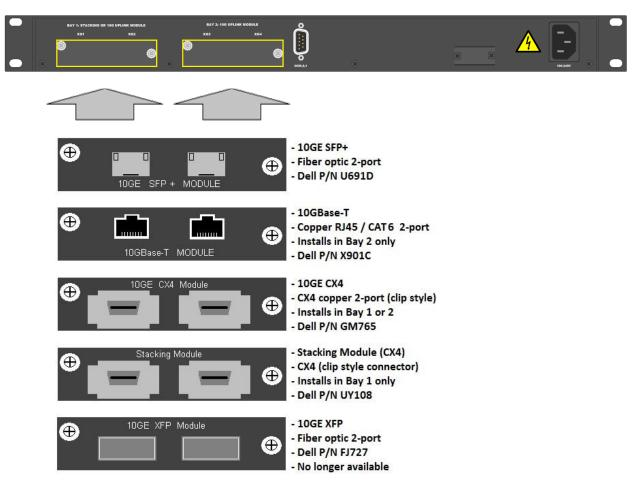
Figure 11 Dell Networking 62xx Series Switch (1G Ethernet) and Available Modules
