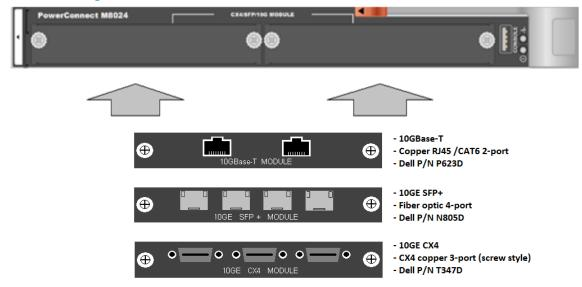
Figure 3 Dell Networking M8024 Blade Switch (10G Ethernet) and Available Modules
