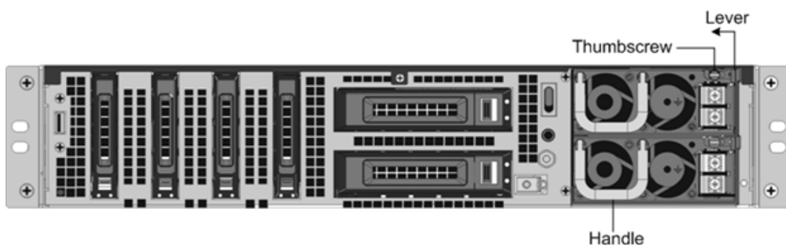
Figure 2. Remove an Existing DC Power Supply
