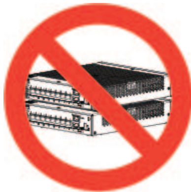
Figure 24: Do Not Stack the Chassis
