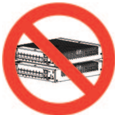
Figure 1: Do Not Stack the ASA Chassis
