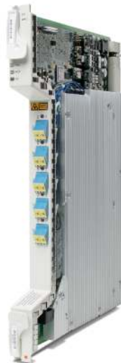
Figure 1. Cisco ONS 15454 Enhanced C-Band Optical Amplifier (OPT-AMP-C)
