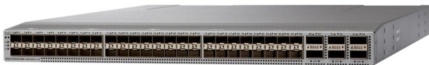
Figure 1. Cisco Nexus 93180YC-EX Switch
