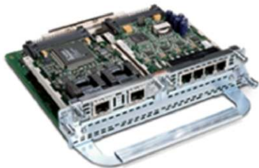
Figure 1. NM-HD-2VE with One VWIC2-2MFT and One VIC3-4FXS/DID
