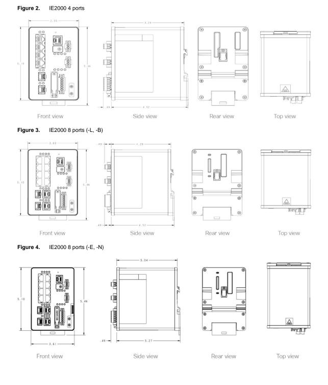
Figures 2–5 show the mechanical dimensions of the various IE 2000 models.
