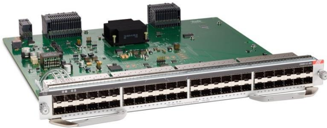
Figure 6. Cisco Catalyst 9400 Series 48-Port 1 Gigabit Ethernet (SFP) Line Card (C9400-LC-48S)
