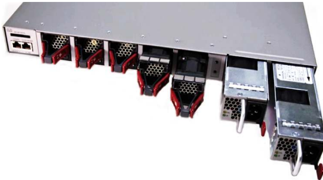
Figure 7. Redundant Fan and Power Supply
