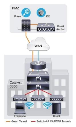
**Figure 11.**Deploying the Cisco Catalyst 3850 Series for branch access
