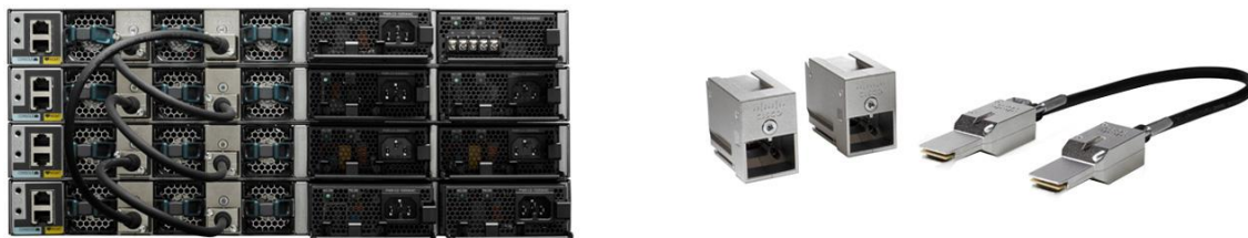
Figure 4. StackWise-160 Kit with Stack Adapters and Cables
