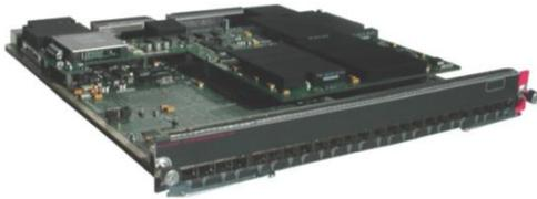
**Figure 4.** 6800 Series 48-Port Gigabit Ethernet Interface Module WS-X6848-SFP-2T/2TXL
