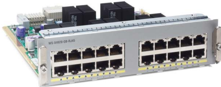
Figure 2. 20-Port Wire-Speed 10/100/1000 (RJ-45) Half Card
