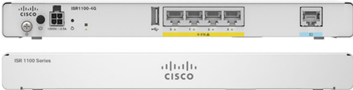
Figure 1. ISR 1100-4G, front and back view
