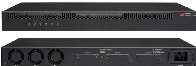
**Figure 3:** The optional Brocade ICX 6400-EPS150 is an external power supply source to provide additional power to the Brocade ICX switches (except the Brocade ICX 6430-C, 6450-C, and 6430-24). It also can be used for system power redundancy and increased PoE/PoE+ power budget to enable additional PoE/PoE+ ports. Each Brocade ICX 6400-EPS150 can connect up to three Brocade ICX 6430 and 6450 Switches.
