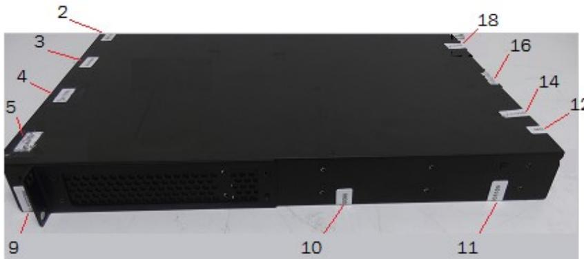
Figure 48 - Right side view of Brocade CES 2024C-4X device with security seals
