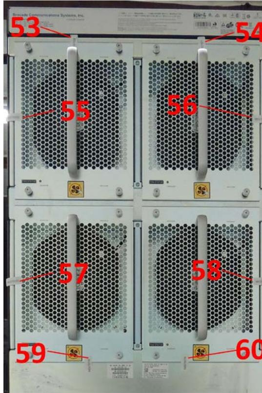
Figure 35 - Back upper chassis of MLXe-32 with tamper labels
