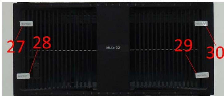
Figure 30 - Front middle chassis (grill) of MLXe-32 Configuration 2 with tamper labels
