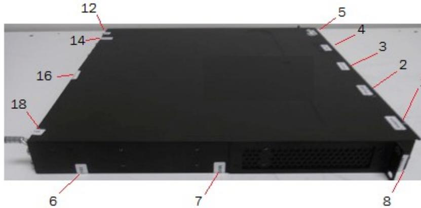
Figure 49 - Left side view of Brocade CES 2024C-4X device with security seals
