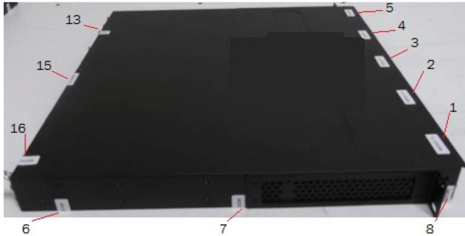
Figure 39 - Left side view of Brocade CER 2024C-4X-RT device with security seals
