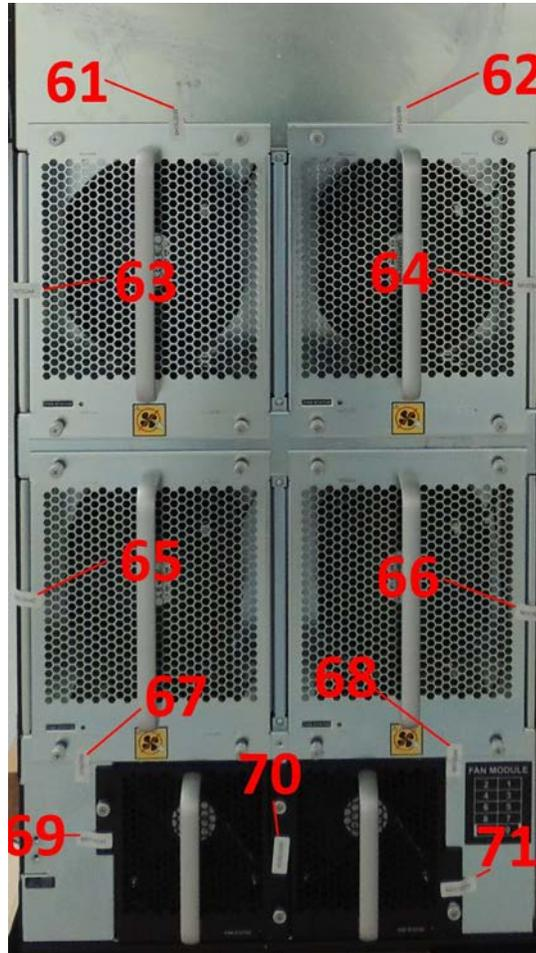
Figure 36 - Back lower chassis of MLXe-32 with tamper labels
