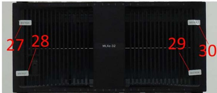
Figure 26 - Front middle chassis (grill) of MLXe-32 Configuration 1 with tamper labels
