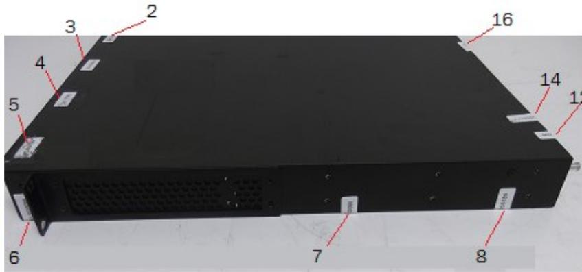
Figure 43 - Right side view of Brocade CER 2024F-4X-RT device with security seals
