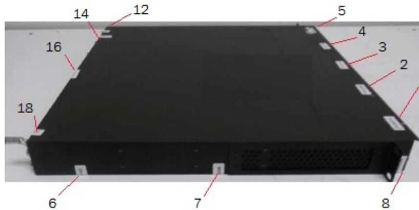
Figure 54 - Left side view of Brocade CES 2024F-4X device with security seals
