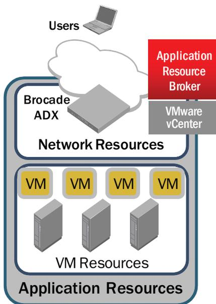
and efficiency to improve overall service availability. ServerIron ADX switches provide highly customizable application-specific health monitoring to help organizations quickly determine any degradation or failure of application servers—and to redirect clients to alternative resources. The frequency of health monitoring messages is user-configurable per server and per application port.
