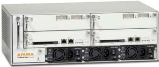
The Aruba 6000 is a modular, full-featured wireless LAN mobility controller that aggregates up to 512 controlled Access Points (APs) and delivers mobility, centralized control, convergence services and security for wireless deployments. The Aruba 6000 is designed to support large deployments in a scaleable manner, and can be easily deployed as an overlay without any disruption to the existing wired network. The
