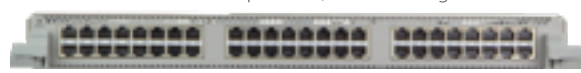
48 port 10GBASE-T line card for 100M/1/10GbE and consistent features - Dense 10G with deep buffers, flexible 100M to 10G mixed speeds
