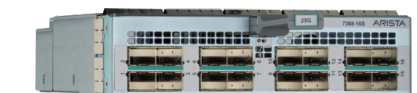
DCS-7368-16S SFP-28 - 16 ports of 25G with support for 25G and 10G on all ports.
