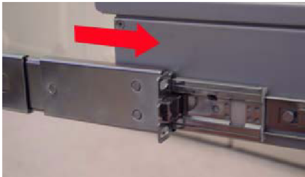
FIGURE 11 Inserting the Server Mounting Brackets Into the Slide Rail Assemblies
