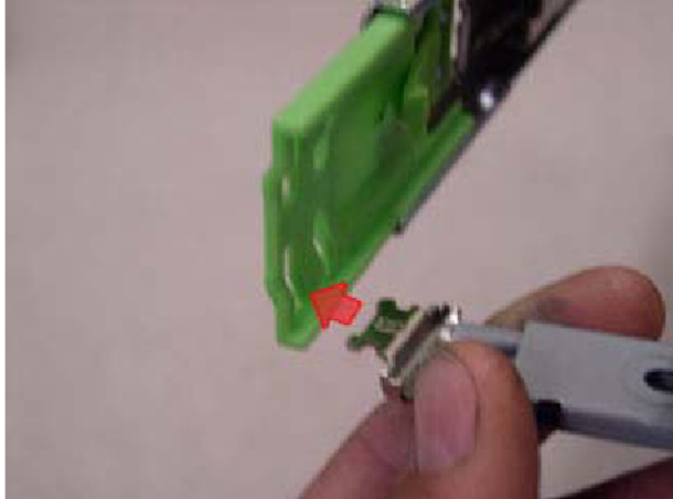
FIGURE 17 Plastic Cutout on Left Slide Rail Extension
