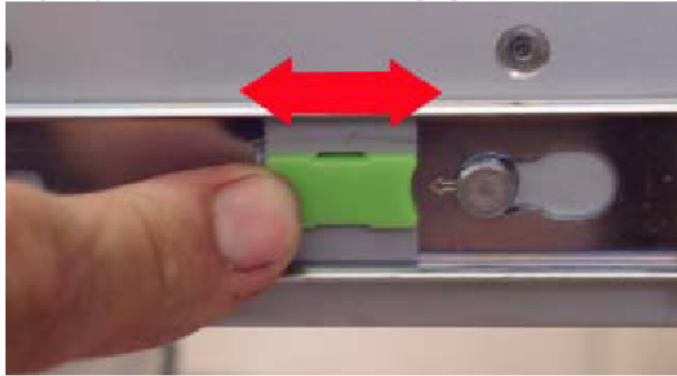
FIGURE 20 Slide Rail Release Button
