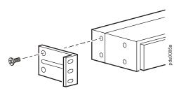
2. Install the PDU using the screws and caged nuts included with your rack or enclosure. The PDU will occupy 1 U-space.
