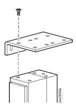
2. Install the PDU on a vertical mounting rail in your rack or enclosure.
